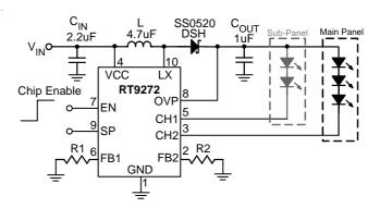
Figure 1. 2LEDs for Sub panel and 3LEDs for Main panel
